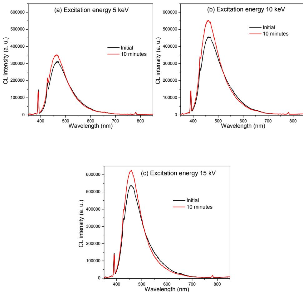
Fig. 14. CL spectra of  $\text{SRO}_{30}$  annealed samples after different times of electron bombardment. Different samples were used: (a) sample excited with 5 keV, (b) sample excited with 10 keV, (c) sample excited with 15 keV.
