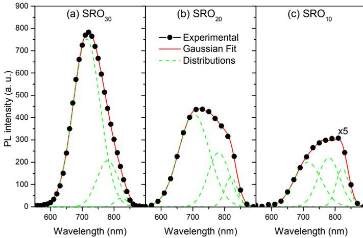
Fig. 7. PL spectra and fits from SRO films with different silicon excess and annealed at  $1100^{\circ}\text{C}$  for 180 min. Symbols are experimental data, lines are the Gaussian fits and dash lines are distributions.
