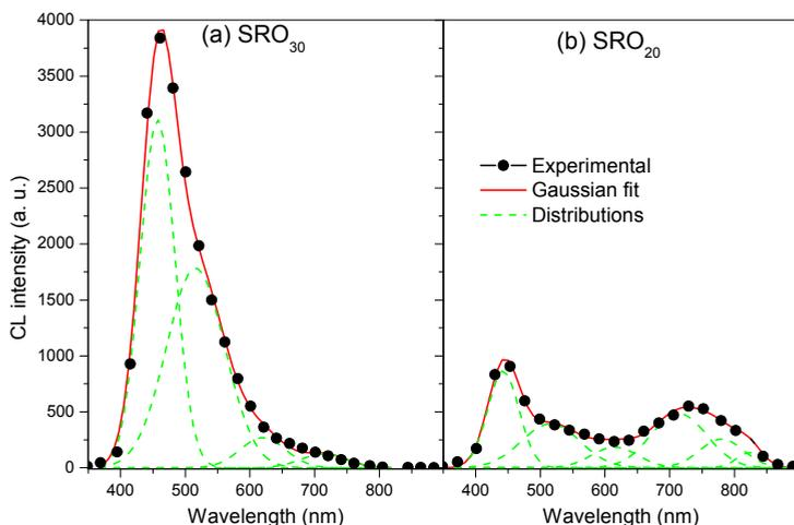
Fig. 9. Gaussian fit of CL experimental spectrum, the best fit requires 4 distributions for (a)  $\text{SRO}_{30}$  and 6 distributions for (b)  $\text{SRO}_{20}$ . Symbols are experimental data, lines are the Gaussian fits and dash lines are distributions.
