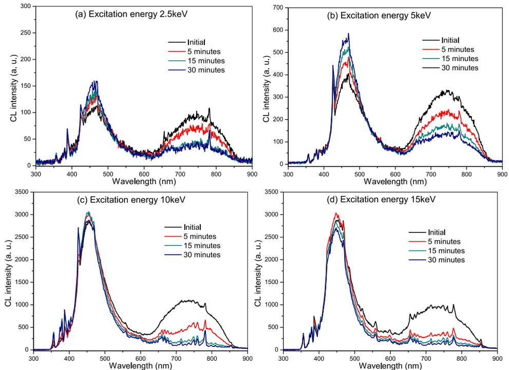
Fig. 12. CL spectra of SRO<sub>20</sub> after different times of electron bombardment. Different samples were used: (a) sample excited with 2.5 keV, (b) sample excited with 5 keV, (c) sample excited with 10 keV, (d) sample excited with 15 keV.
