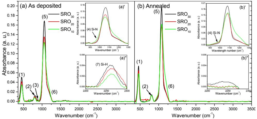
Fig. 1. FTIR absorption spectra of SRO films with  $R_0 = 10$  (a) before and (b) after thermal annealing. The inset shows Si-N and Si-H bonding in the 850 to 1300  $\text{cm}^{-1}$  and 2200 to 2300  $\text{cm}^{-1}$  range.
