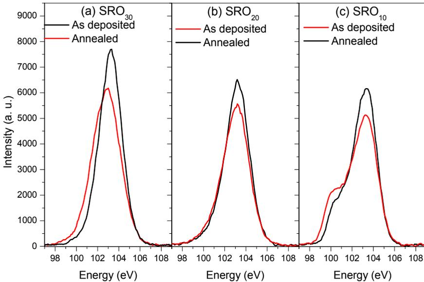
Fig. 3. Si 2p XPS peaks for as deposited and annealed samples with different flow ratio (R<sub>0</sub> 30, 20 and 10).
