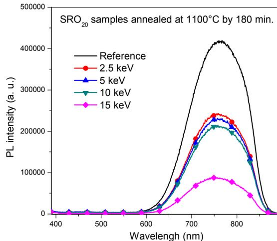
Fig. 13. PL spectra of SRO<sub>20</sub> samples after continuous cathode-excitation during 30 minutes. Solid line is the reference sample emission (without electron beam irradiation). The symbols represent the PL emission after cathodo excitation.
